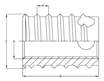
Female thread A = M24 Length B = 30 Male thread E = 30 Min hole depth blind hole = 34 Thread pitch P = 2
